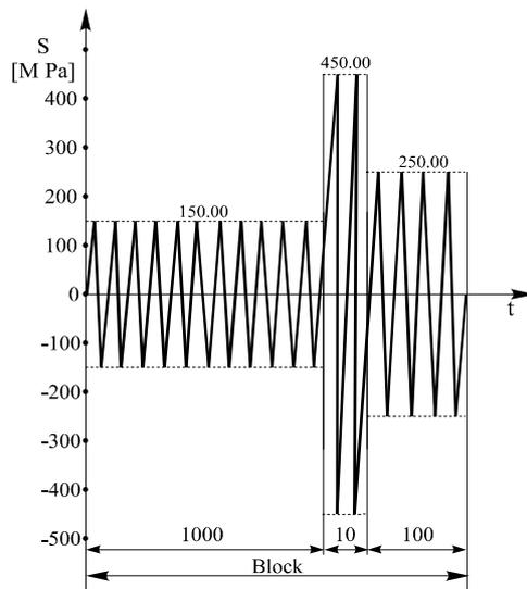
**Figure 3.** Load spectrum
