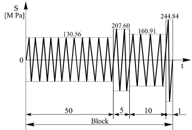
Figure 7. Load spectrum
