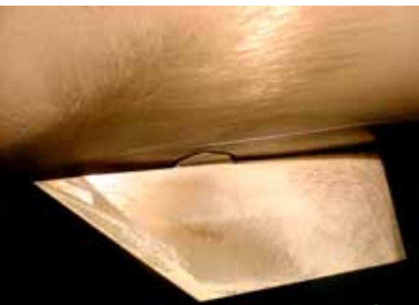
Figure 11. Flow on the fin upper surface, RSN=46
