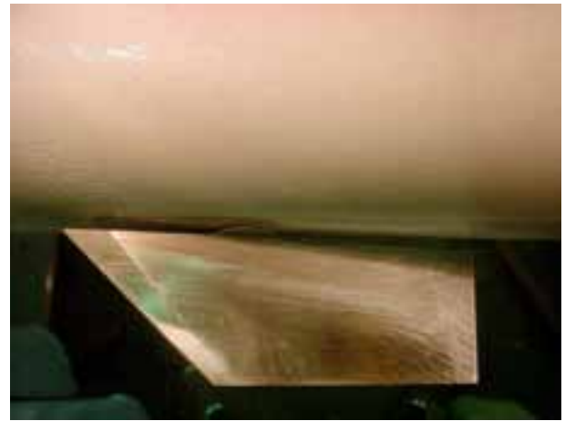
Figure 12. Flow on the fin upper surface, RSN=47
