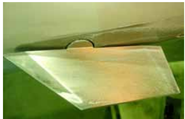
Figure 15. Flow on the fin upper surface, RSN=50
