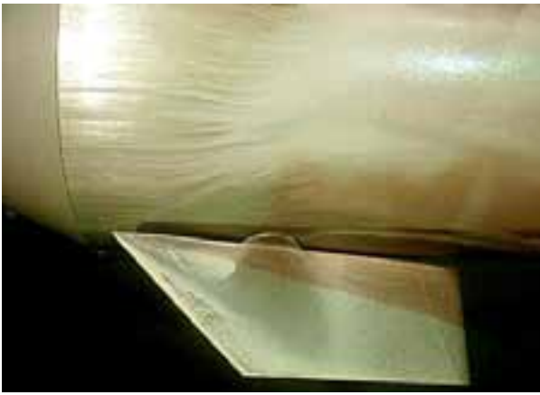
Figure 8. Flow on the fin upper surface, RSN=43
