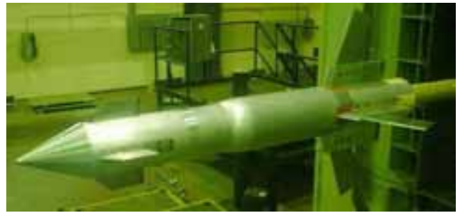
Figure 3. Basic configuration of the LGB model in the T-38 wind tunnel test section
