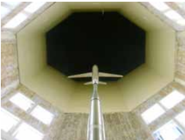
Figure 4. ONERA M4 calibration model on the model support system in the wind tunnel T-35 test section
