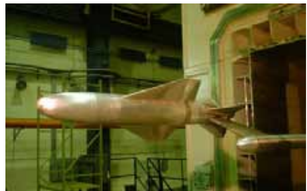
Figure 5. P22 model in the test section of the T38 wind tunnel
