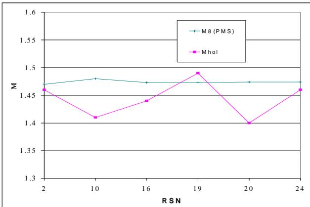
Figure 5. Determination of Mach number  $M_\infty$  by angle of shock wave
