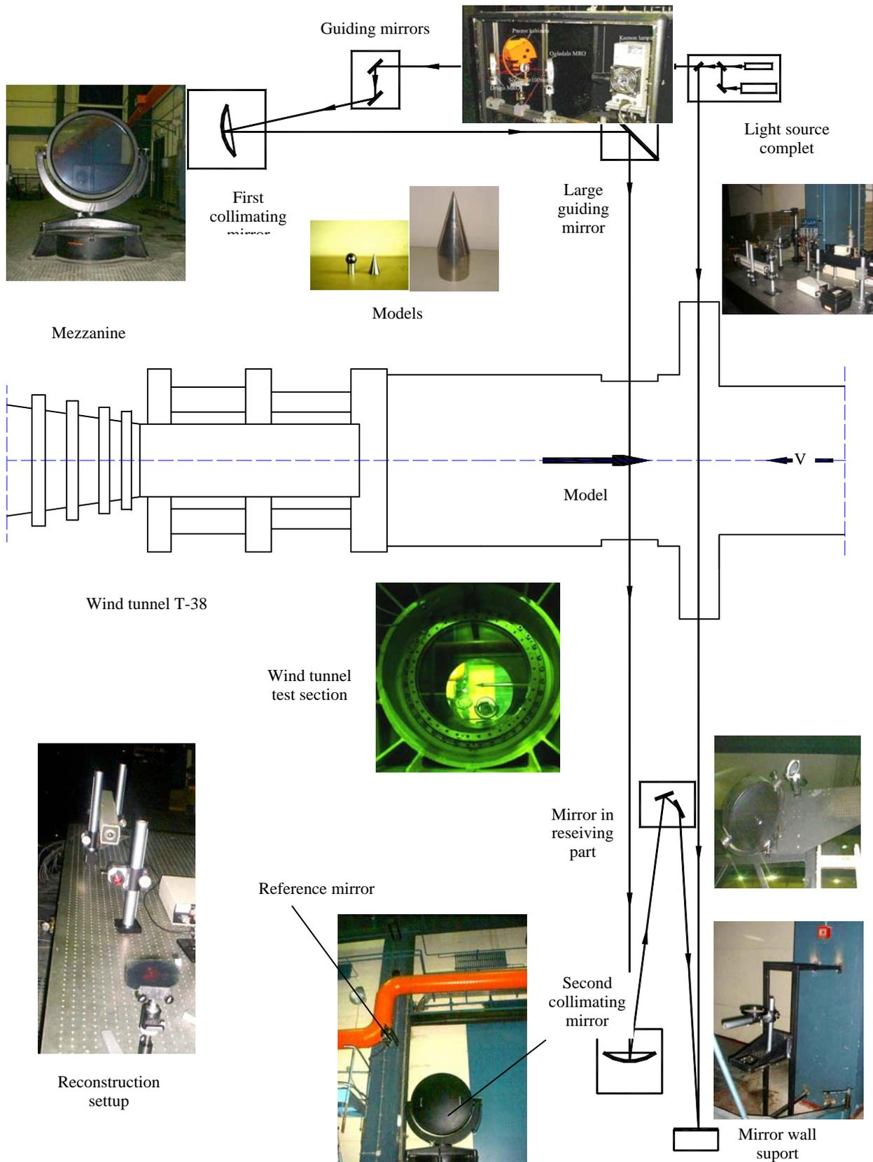
Figure 1. The holographic interferometer in wind tunnel T-38 (top view)
