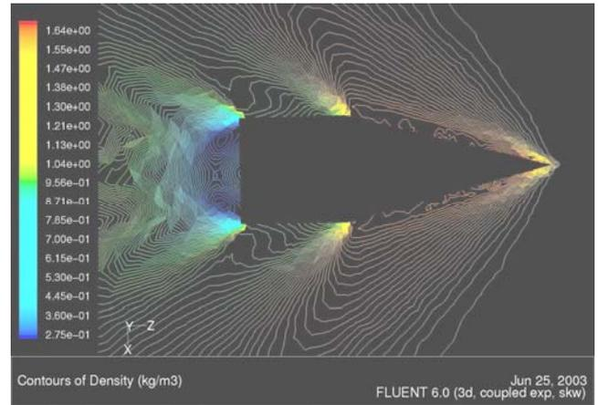
Figure 7. Theoretical simulation of isodensity lines of flow around model cone-cylinder with  $M_\infty = 1.474$  (M.Zdravković [18])
