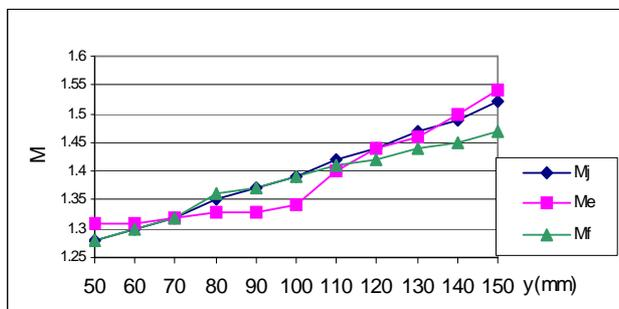
**Figure 4.** Mach number behind shock wave for  $x=150\text{mm}$ ,  $y=50-150\text{mm}$
