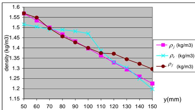
**Figure 3.** Experimental density distribution behind shock wave
