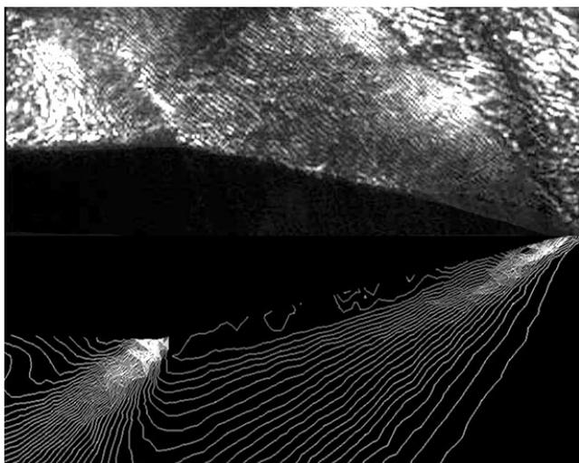
**Figure 8.** The composite experimental and theoretical image of flow isodensity lines
