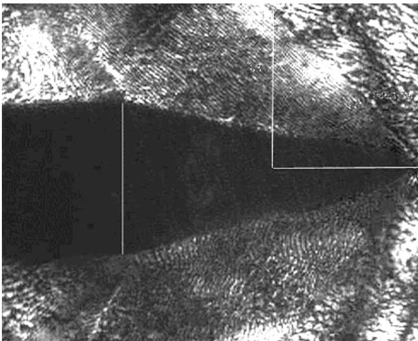
Figure 6. Interferogram of flow around model cone-cylinder with  $M_\infty = 1.474$  ( $RSN=20$ )
