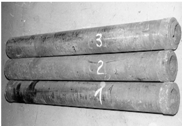
Figure 1. The centrifugally cast Cr-Mo-V steel tubes A
