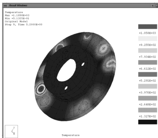
Figure 17. Temperature fields in the moments t=5.2 and t=45 s respectively
