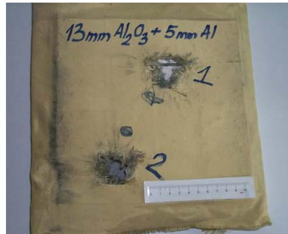
**Figure 2.** Facing side of the composite ceramics/Al-alloy armour after ballistic tests
