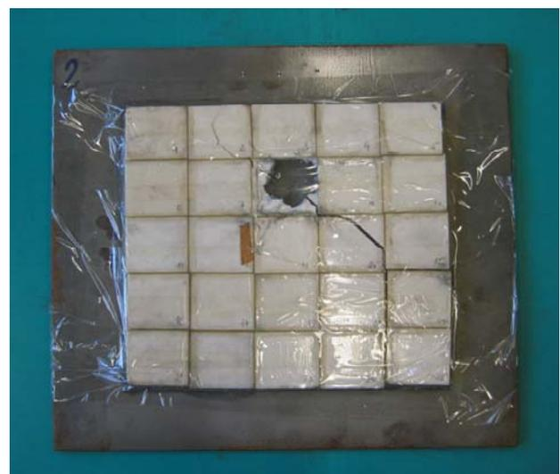
**Figure 3.** Facing side of the composite ceramics/armour steel armour after ballistic tests
