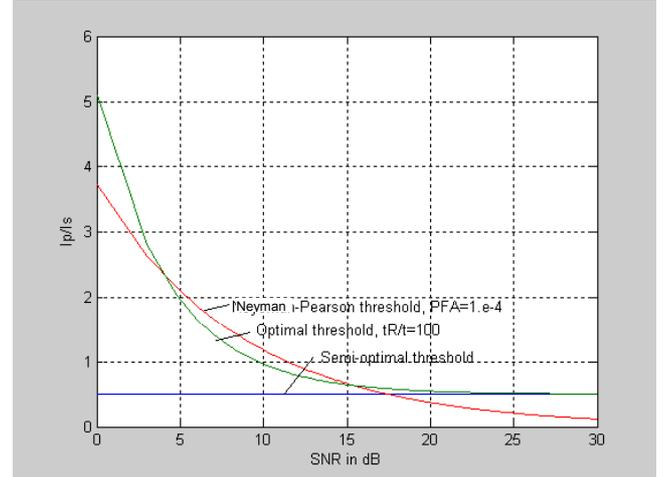
Figure 4. Ratio  $I_p/I_s$  as a function of the SNR
