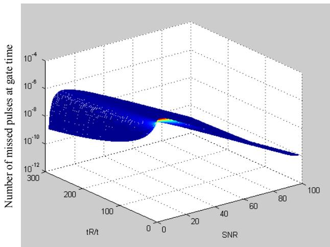
**Figure 7.** Number of missed pulses as a function of both SNR and  $t_R/\tau$ , for  $t_R/T_i=1.0e^{-3}$
