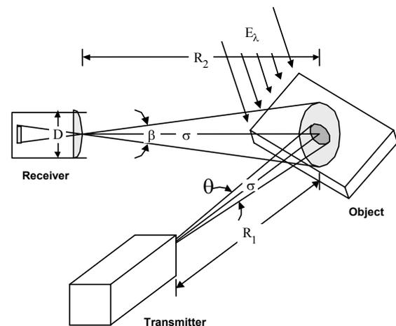
Figure 1. Block diagram of a pulse laser tracking system
