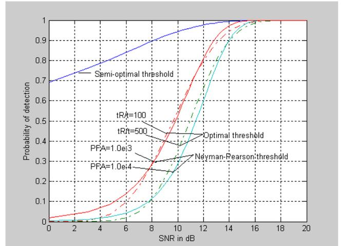
**Figure 9.** Probability of detection as a function of the SNR
