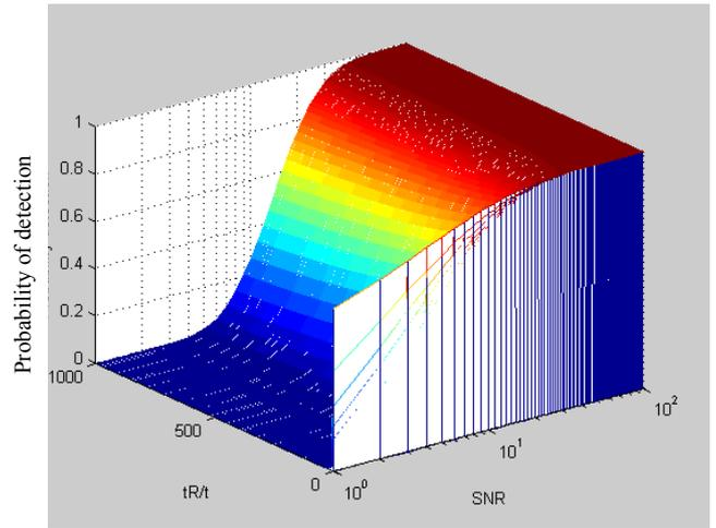
**Figure 8.** Probability of detection as a function of both SNR and  $t_R/\tau$
