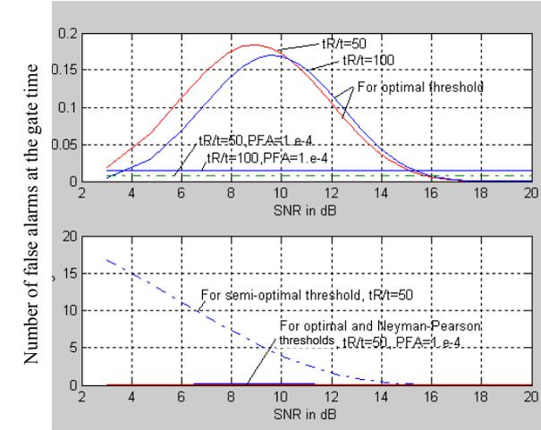
**Figure 6.** Number of FAR as a function of the SNR, for the parameters  $t_R/\tau=50;100$ , and  $P_{FA}=10^{-4}$
