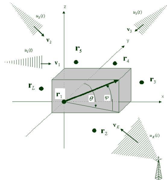
**Figure 1.** Superposition of radio signals on the antenna array of arbitrary volume non-uniform geometry
