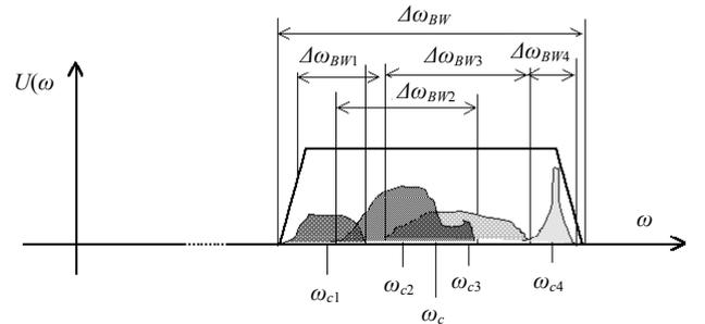
Figure 2. Superposition of radio signals in a given frequency sub-band
