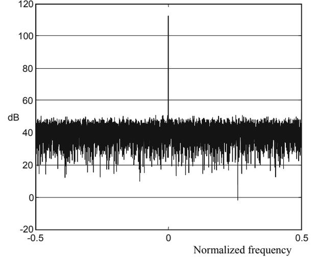
Figure 8. Amplitude spectrum of the baseband signal calculated by the FFT
