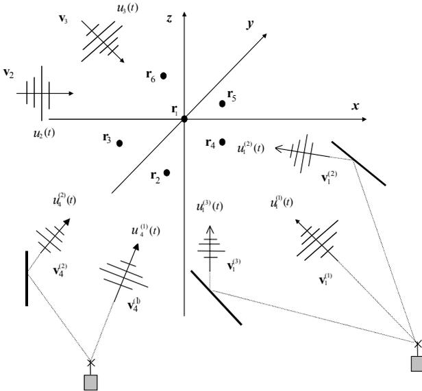
Figure 3. Superposition of radio signals under multipath conditions
