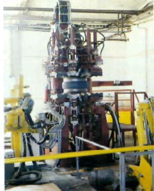
Figure 3. Machine for the production of LIM tires a complete control over the process of producing tires for passenger vehicles by liquid injection moulding
