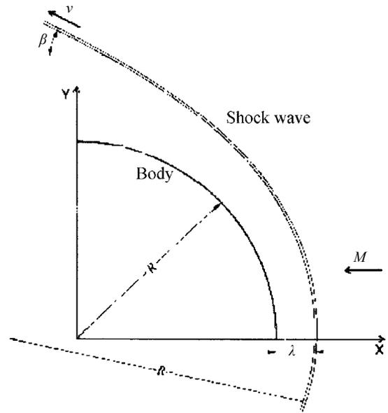
Figure 1. Coordinate system and variables in Billig's equation
