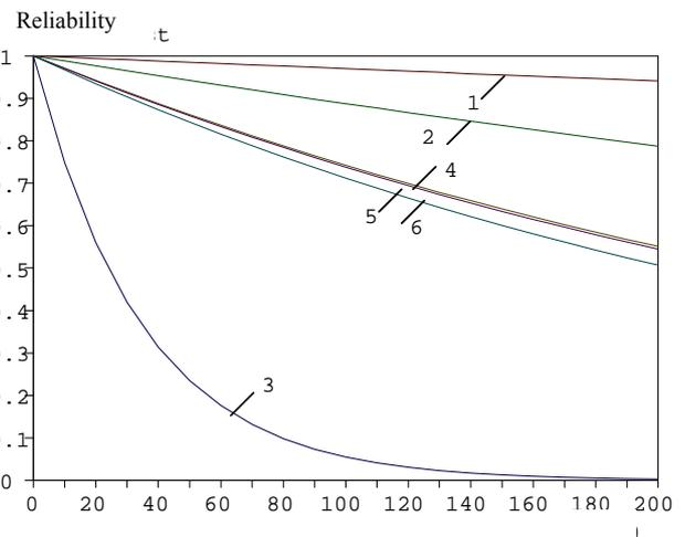
**Figure 7.** Reliability versus time for the redundant system
