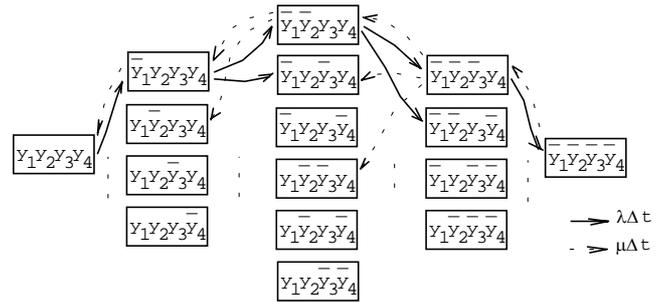
Figure 5. States of the telecommunication system in the first group of the fifth state
