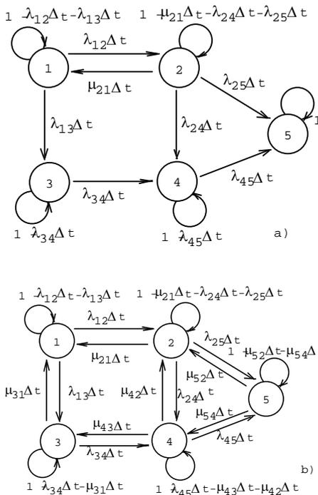
Figure 2. Reliability (a) and availability (b) diagram for the system in Fig.1
