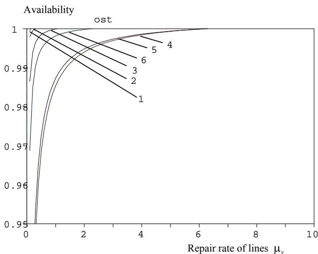
Figure 11. System availability versus the line repair rate
