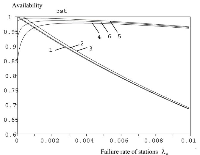
**Figure 8.** System availability versus the station failure rate
