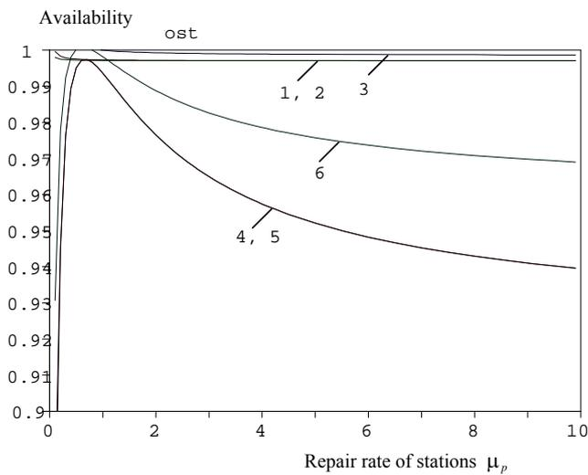
Figure 10. System availability versus the station repair rate
