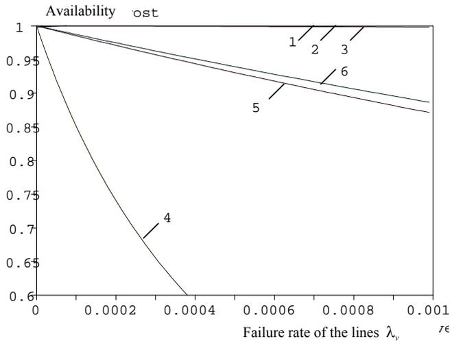
Figure 9. System availability versus the line failure rate
