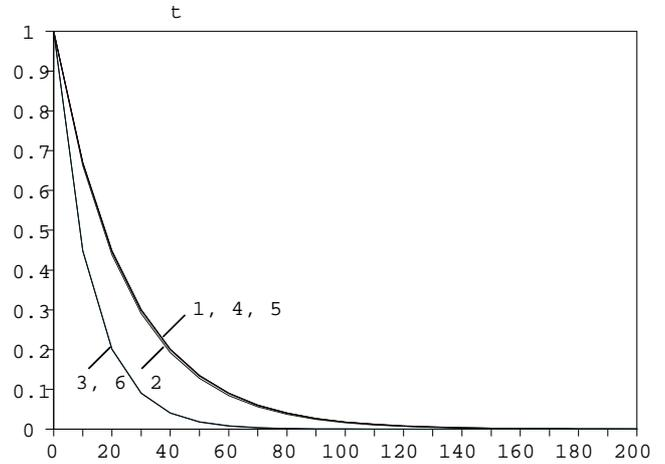
**Figure 6.** Reliability versus time for the unredundant system
