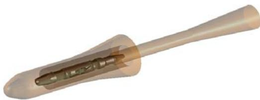
**Figure 1.** Sting, balance and the model installation
