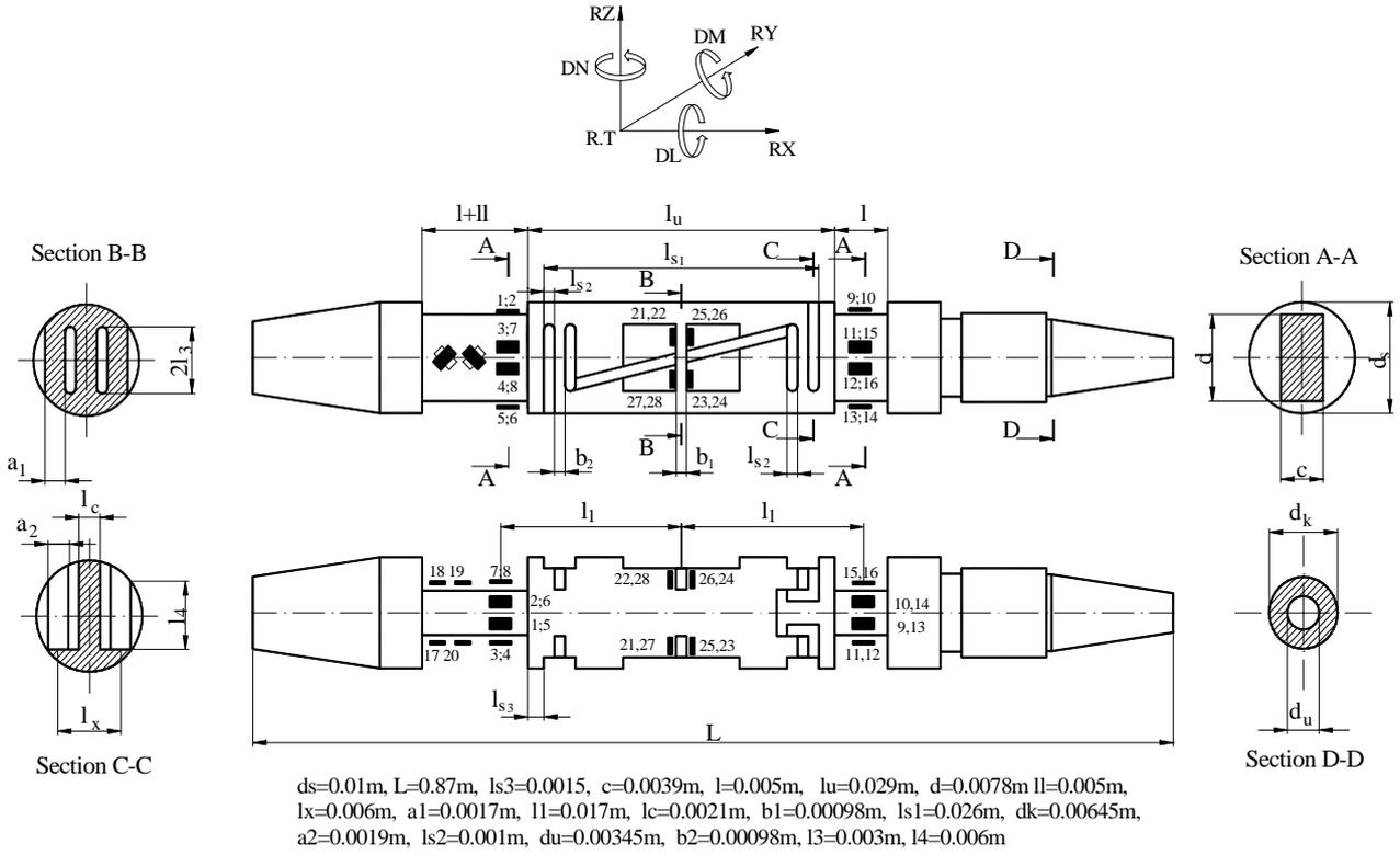
Figure 3. Internal six-component strain gauge balance VTI-10C
