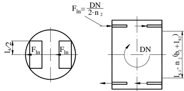
Figure 10. Components of the yawing moment
