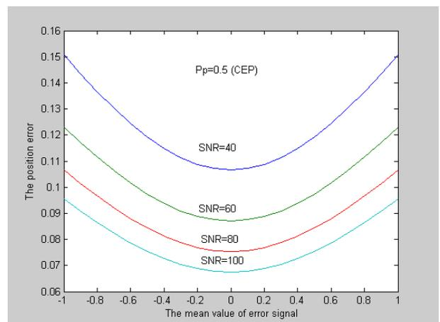
Figure 6. The position error as a function of the mean value, for the positioning probability of 50% and the signal-to-noise ratio as a parameter  $SNR=40, 60, 80$ , and  $100$ .
