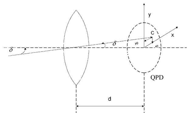
Figure 1. The geometry between the thin lens and the quadrant photodiode
