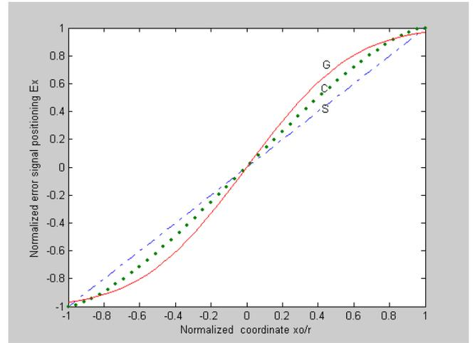
Figure 3. Normalized error signal  $\varepsilon_x$  as a function of displacement of the spot center and the photodiode center, for the constant (S-square, C-circle spot shape) and the Gaussian distribution (G) of irradiance on the photodiode surface
