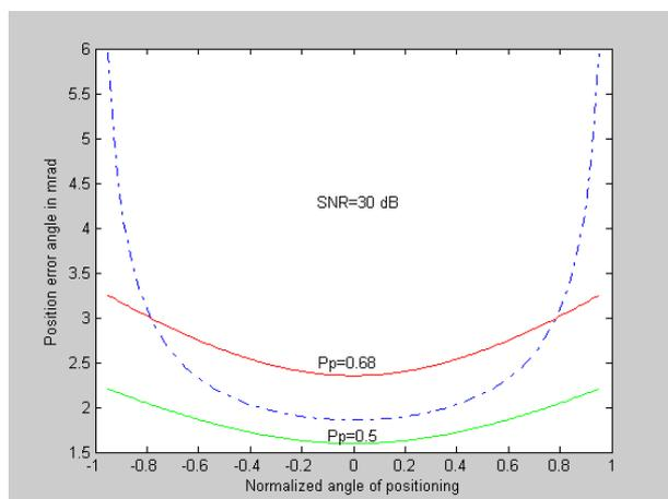
**Figure 7.** Position error angle as a function of the angle of positioning; deterministic (-) and statistics approach for:  $P_p=0.5$  and  $0.68$ ,  $SNR=1000$ ,  $r=2.25$  mm, and  $d=30$  mm
