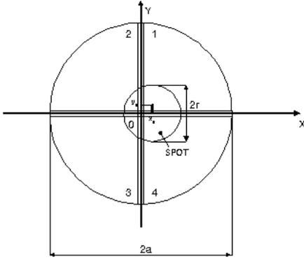
Figure 2. A spot position on the quadrant photodiode surface
