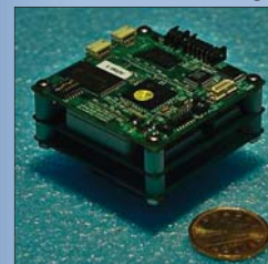
Quality Miniature Video Engine for High End Thermal Imaging Cameras.
